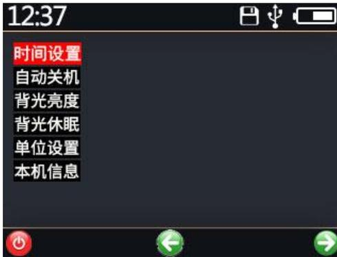
"Time setting": used to set the current time. Generally, it does not need to be set. It has been automatically calibrated at the factory.
