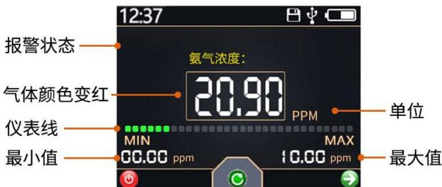
Under the single gas display interface, short press the "left turn page/cancel key" can realize the function of clearing the statistics of the maximum and minimum values, and at the same time, the sound and light alarm can be eliminated in the alarm state.
