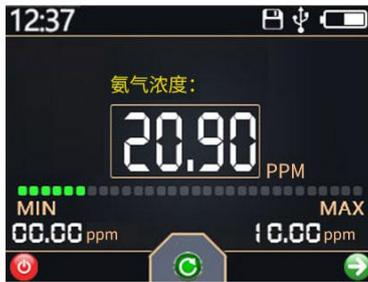
In the all-in-one gas interface, short press the "right turn page/confirm button", automatically jump to the single gas display interface, the single gas display interface will only display a certain gas, but the data shown are more comprehensive.
