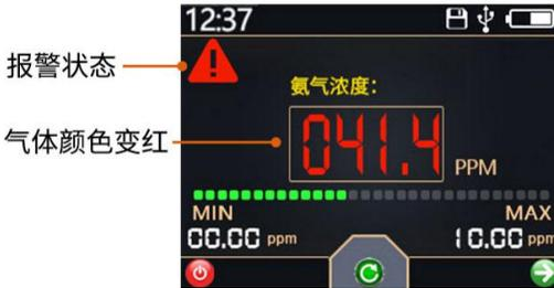
In the alarm state, short pressing the "page left/cancel button" will cancel the alarm and turn off the alarm state of the buzzer and alarm light, but the red number and alarm icon on the screen will not disappear. If another gas triggers the alarm again in the alarm state, the buzzer and the alarm light will still indicate the alarm until the alarm is lifted or the alarm is manually eliminated.
