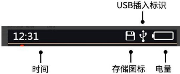
12:31 on the left side of the status bar is the current time, and the current time is 12:31. There are three icons on the right. The first icon is the storage icon. The icon appears after the storage function is turned on. The icon will automatically turn green every time it is stored. When the storage space is insufficient, the icon will turn red.
