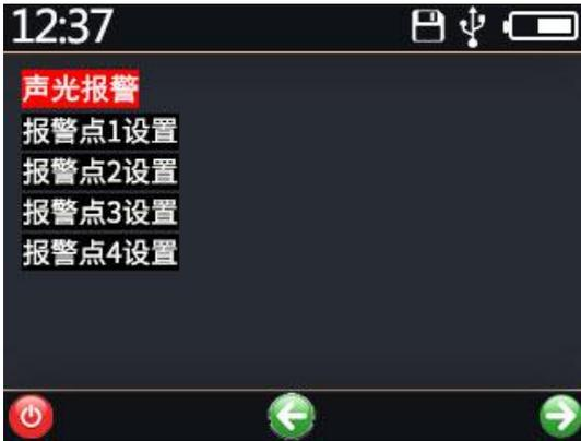
Among them, "sound and light alarm" is used to set whether to turn on the sound and light alarm, the degree of alarm sound after turning on the sound and light alarm, set 0 to turn off the sound and light alarm, and 1-5 represents different emergency procedures, the sound of 1 is the most compact, and the sound of 5 is longer.
