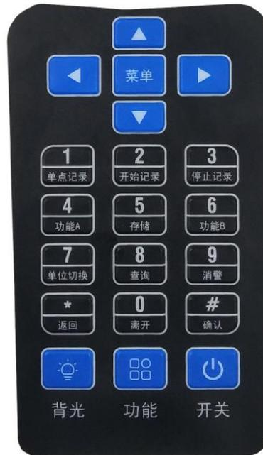
The area above the keyboard is "menu key" and "top, bottom, left, right key ", a total of 5 keys.
